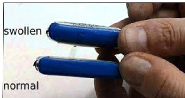
Fig. 2.3.1. Bulging of battery
